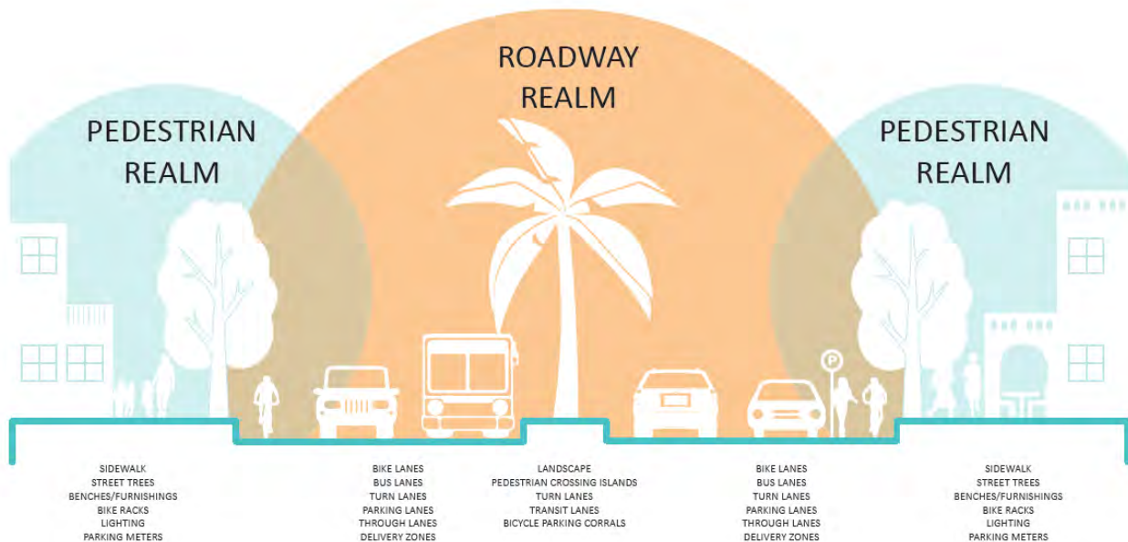
Figure 6: Complete Street Cross Section Elements
